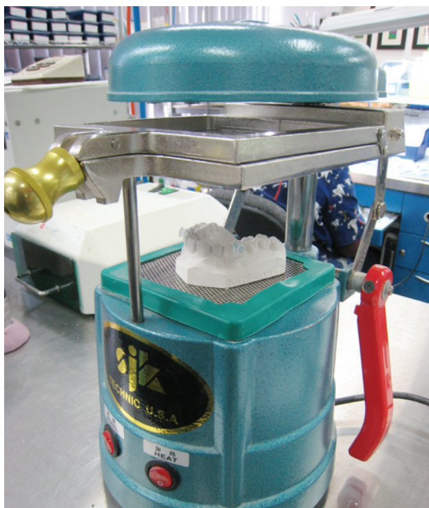
Figure 7. Use a vacuum- or pressure-forming machine to form the material over the model and lugs. The material will form well over the lugs due to the nature of the proprietary thermoforming plastic.
